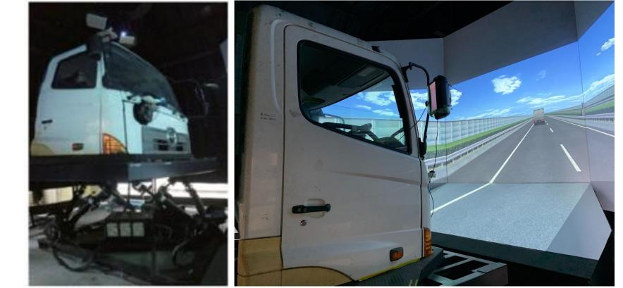
The truck cabin is installed on a 6-degree-of-freedom motion platform. A four-sided screen is in the front including the front lower one. Using a truck model (Gross Vehicle Weight: 24 t).
