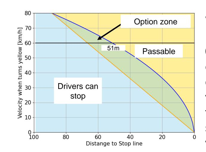
When Vehicle deceleration is 3.0 m/s<sup>2</sup> and ADAS reaction time is 0.3s are assumed, there are only optional zones where the vehicle can stop and pass through at a yellow light. There are cases where the ADAS judges the vehicle can stop, but the driver judges the vehicle can pass through.
