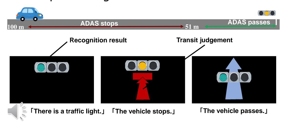
HMI which cannot present the detection failure
