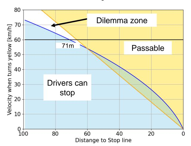
When Vehicle deceleration is 3.0 m/s<sup>2</sup> and driver reaction time is 1.5s are assumed, there are optional zones where the vehicle can stop and pass through at a yellow light, and dilemma zones where neither is possible.
