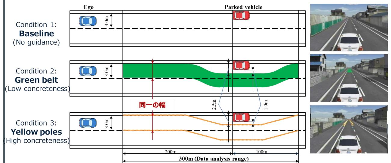
To investigate correlation of concreteness of visual information (accuracy of tracing specified route) for overtaking assistance and safe driving performance, we conducted a driving simulator experiment.
