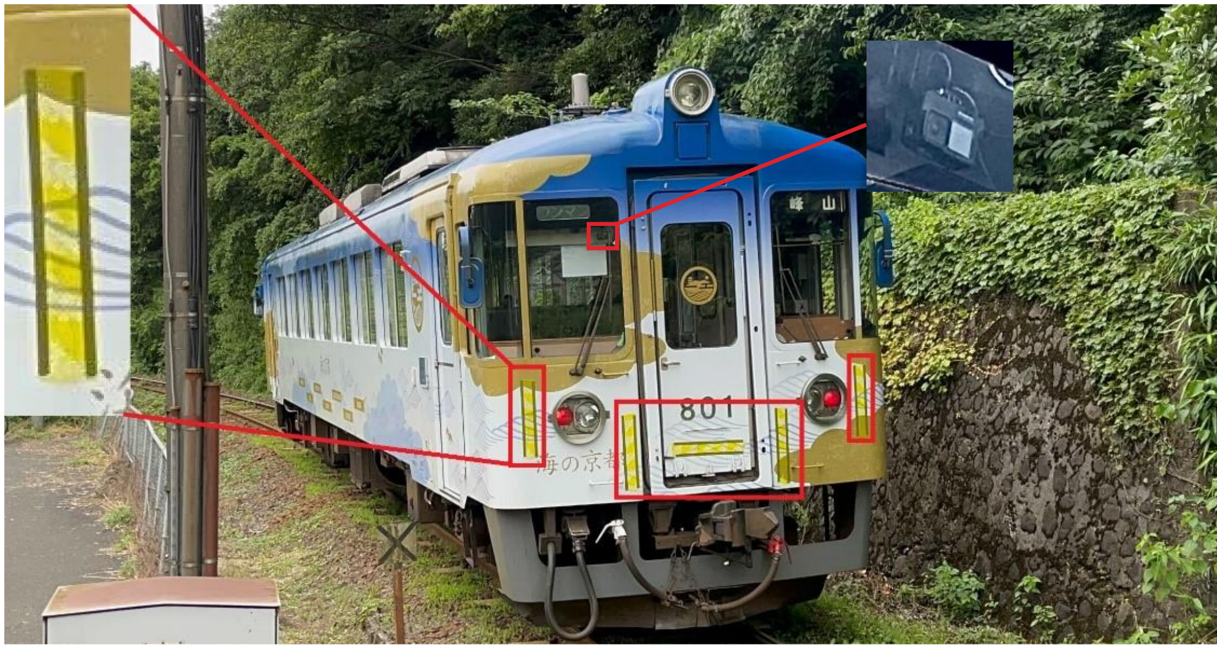
A rolling stock in normal service with tapes and cameras applied
