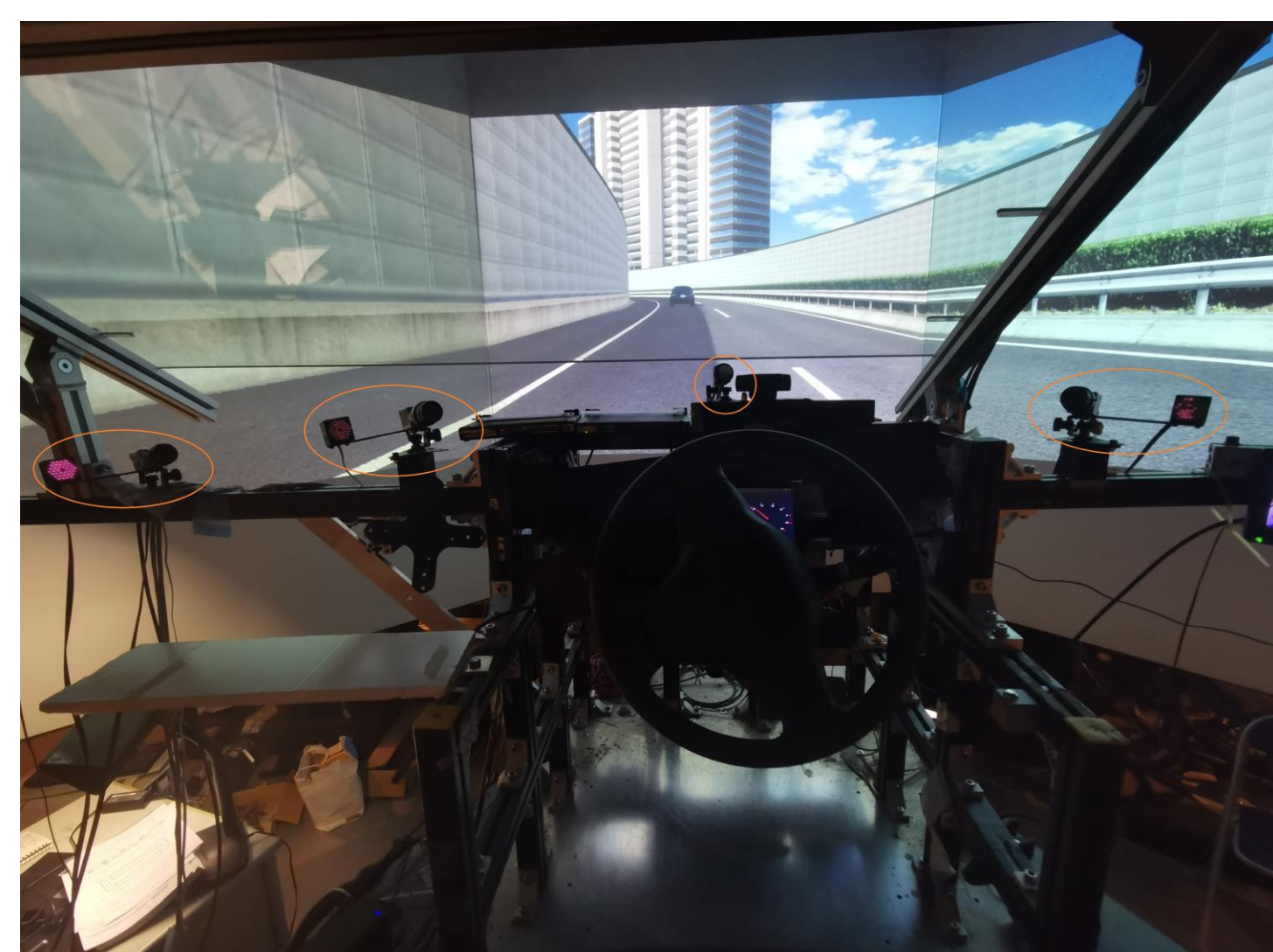
Fixed driving simulator and Smart Eye Pro eye tracking system.
